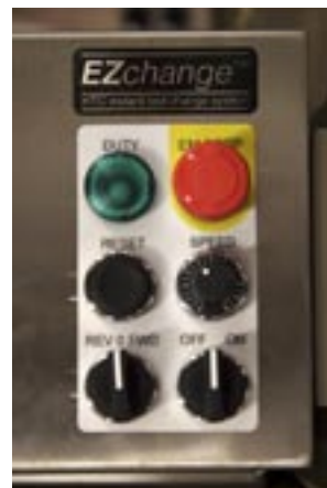
Control panel for frequency controlled machine
