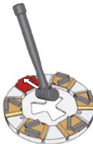
Picture 2. Now you can lock the tool in the tool holder by applying a few light blows with a rubber hammer.
