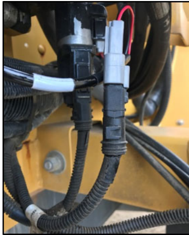
Figure 12: Cable C11 Connection to Directional Coil
