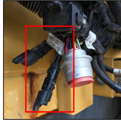
Figure 15: Cable C30 CAN Connection
