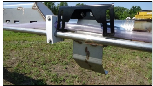
Figure 8: Remove Bolts from Skid Plate and Use to Mount Bracket Adapter
