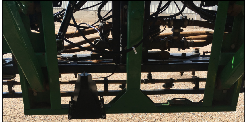
Figure 17: Example Mounting of the Main Lift Bracket
