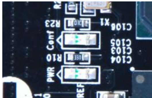
Figure 8-2: Power Indicator and Configure Indicator on the Core Board
