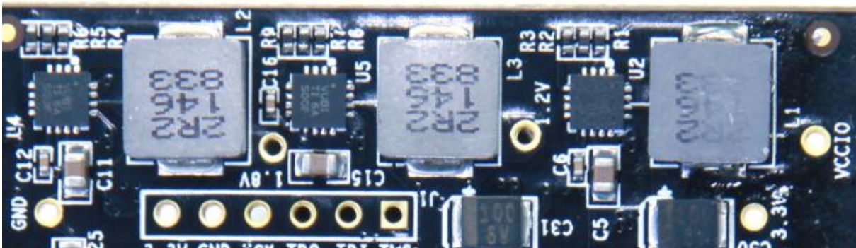
Figure 4-3: Power Supply Circuit on the Core Board
