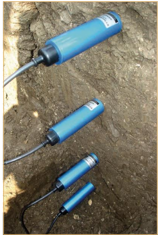
MP406's installed down a soil column
