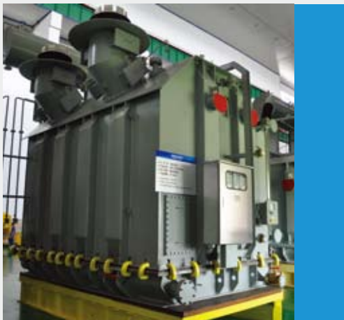
沈变——糯扎渡水电站 DSP-241MVA/500KV Shenyang transformer-Nuozhadu hydropower station DSP-241MVA/500KV
