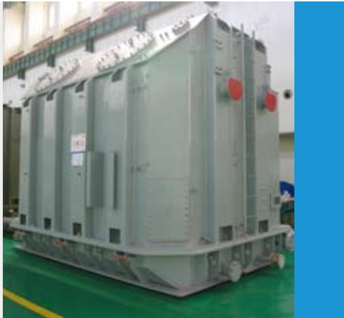
沈变——小湾电厂 DSP-260MVA/500KV Shenyang transformer-Xiaowan power plant DSP-260MVA/500KV
