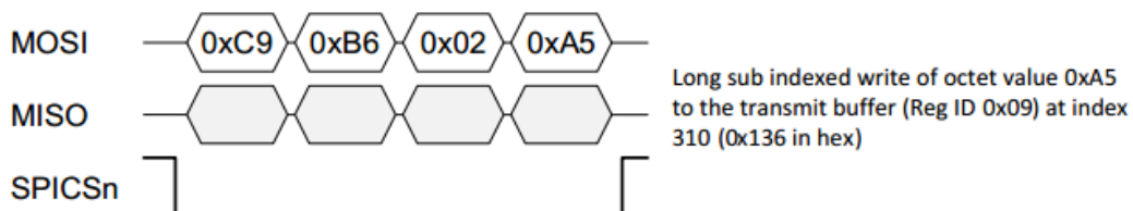
Figure 7: Example long-indexed write of one octet to index 310 of the TX buffer
