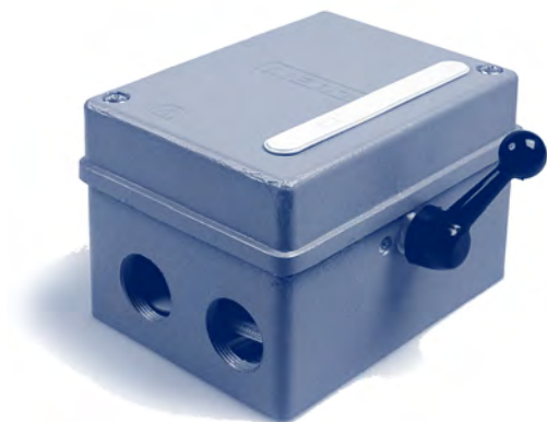
Lever on/off switch in watertight enclosure IP54 with PG16 entries
