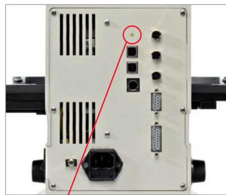
The service LED indicates the service status.
