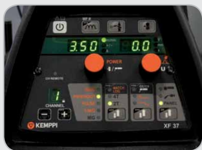
XF 37 control panel of the MXP 37 Pipe wire feeder.
