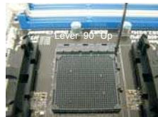
STEP 1: Lift Up The Socket Lever
