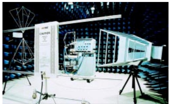
EMC Radiation testing
