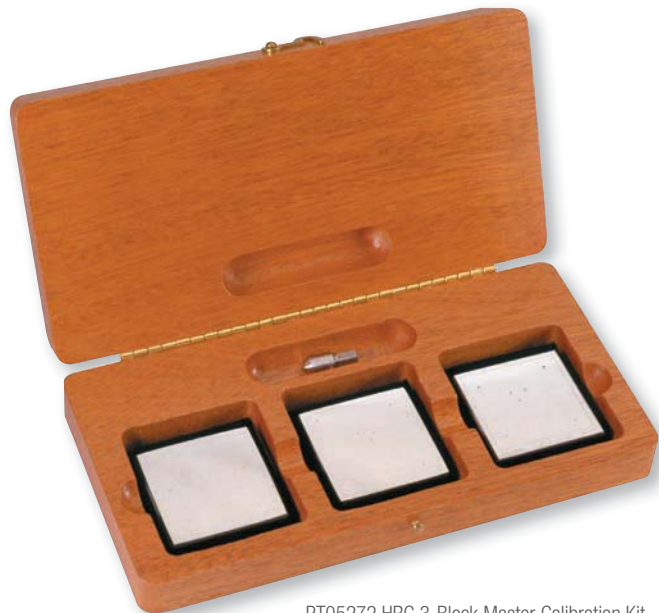
PT05272 HRC 3-Block Master Calibration Kit
