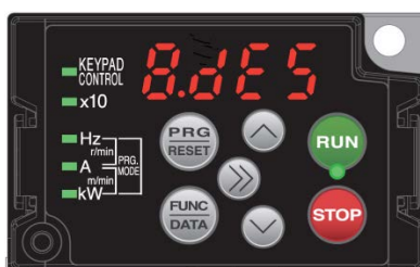
Figure 4.3-1 Display of the LED Monitor after Power-on
