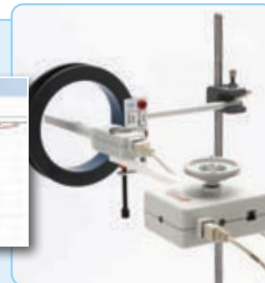
Variation in magnetic field strength along the axis of a coil.
