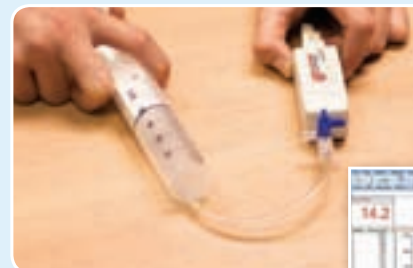
A very simple way of investigating Boyle's Law. The sensor records the pressure in the plunger as the syringe is released.
