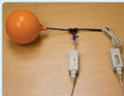
This temperature probe is ideal for measuring the temperature in confined spaces. Here it is shown in a Charles Law experiment.
