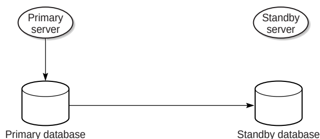
Figure 13 Server and database roles before database switchover
