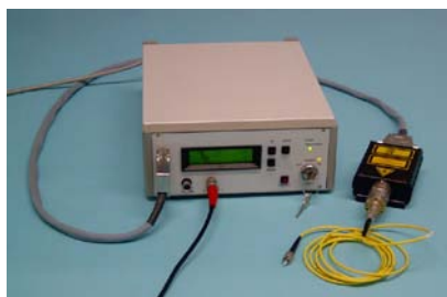
EIG1000D with PIL063G/XS 8 (fiber coupler and fiber)
