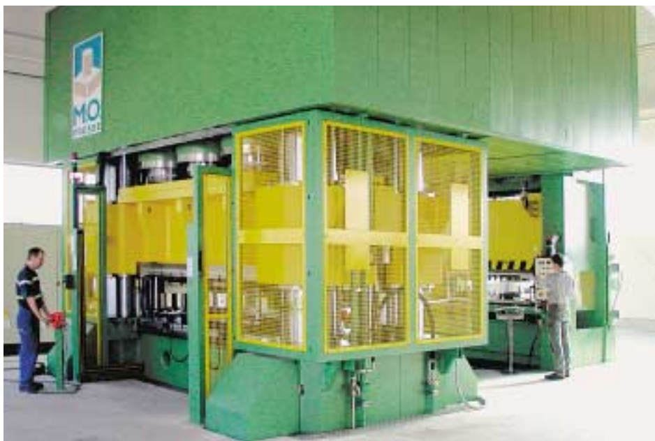
Embossing of quality plates with 6000 tons clamping force
