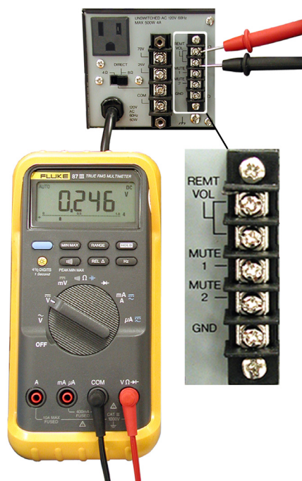
Figure 2-7 — Measuring control voltage for a TOA A-903 amplifier
