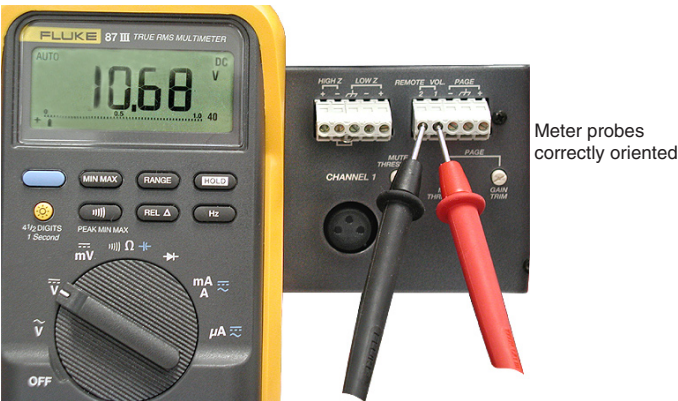
Figure 2-3 — Measuring control voltage for a Peavey UMA 35T II: Meter probes are oriented correctly.
