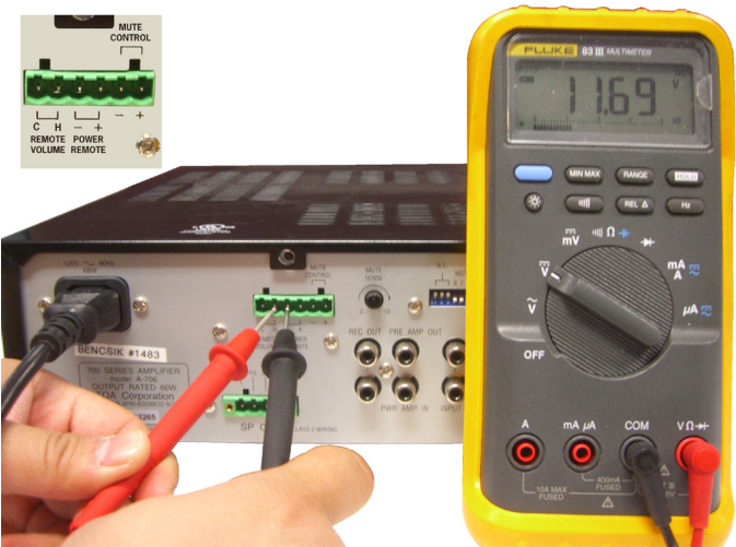
Figure 2-6 — Measuring control voltage for a TOA A-706 amplifier
