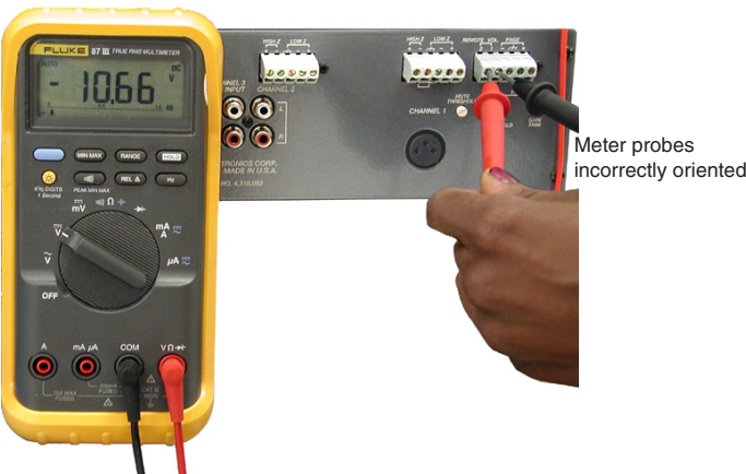
Figure 2-4 — Measuring control voltage for a Peavey UMA 35T II: Meter probes are oriented incorrectly.
