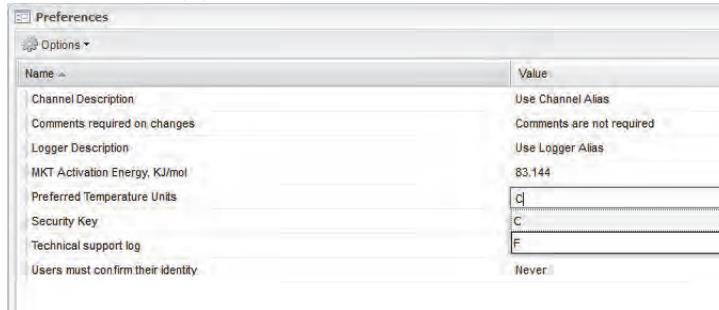
**Note:** This procedure does not alter how the device measures temperature - it alters the units in which temperature is displayed (except for channels which already have preferred unit settings assigned).
