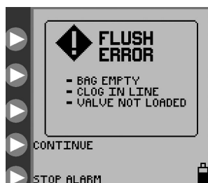
Figure 29. Flush Error screen.
