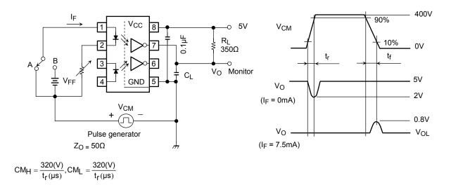
$^{\ast}$  CL is approximately 15pF which includes probe and stray wiring capacitance.
