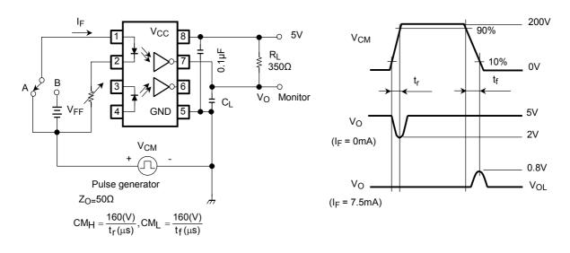
$^{\star}$   $\,$   $\,$   $\,$   $\,$  C  $_{L}$  is approximately 15pF which includes probe and stray wirng capacitance.
