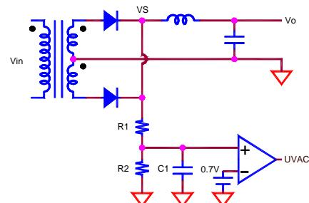
capacitor must be connected between UVAC and ground to filter the switching noise.
