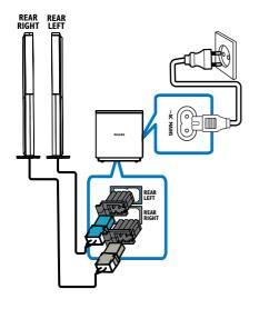
Connect the speaker adapters, rear left, and rear right speakers to the matching connectors at the bottom of the wireless receiver.
