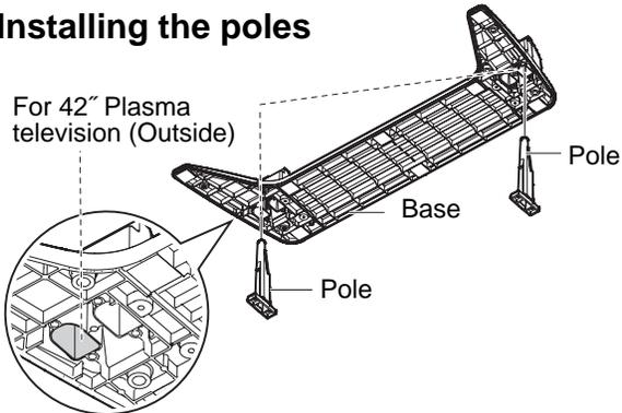
Insert the poles into the left and right holes in the underside of the base so that they fit securely as shown in the illustration above.
