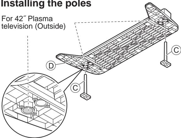
Insert the poles Ⓒ into the left and right holes in the underside of the base Ⓓ so that they fit securely as shown in the illustration above.
