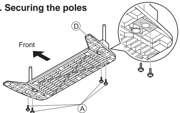
Use the assembly screws Ⓐ to secure the poles firmly to the bottom of the base.
