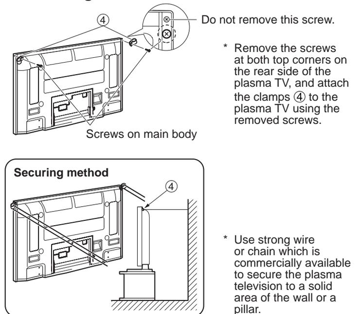
\* The plasma TV must be fastened to both the base and the wall.
