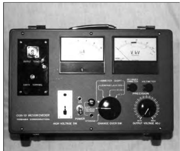
Fig. 33 Toshiba Portable Vacuum Checker
