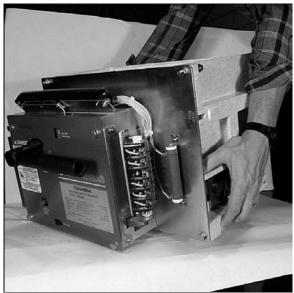
Fig. 7 Correct Method for Handling the ML Type Circuit Breaker
