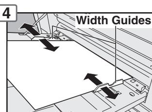
Adjust the width guides. Incorrect adjustment may cause the paper to wrinkle, misfed, or skew.
