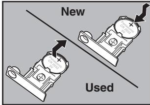
“+” side of battery should be facing upwards.
