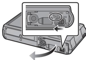
**2** **Battery:** Being careful about the battery orientation, insert all the way until you hear a locking sound and then check that it is locked by lever (A). Pull the lever (A) in the direction of the arrow to remove the battery.
