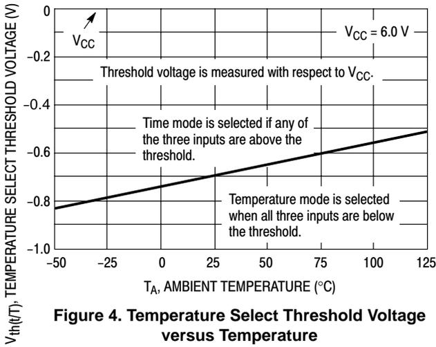
**Figure 4. Temperature Select Threshold Voltage versus Temperature**
