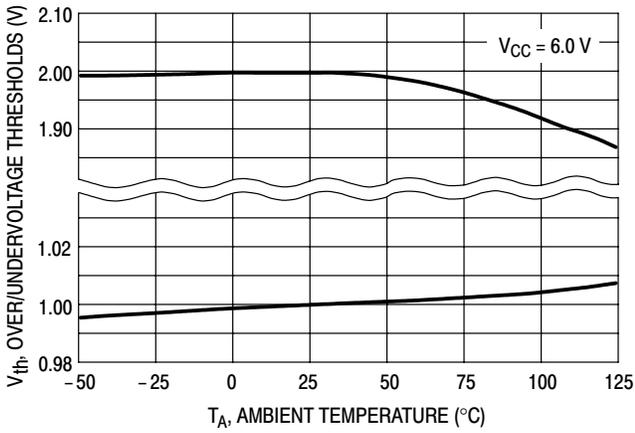
**Figure 2. Battery Sense Input Thresholds versus Temperature**
