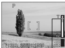
The cursor moves up and down on the zoom indicator according to the zoom magnification. The cursor turns orange when inside the digital zoom area.
