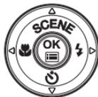
The Arrow pad can be used to set the macro mode, flash mode, and other settings. It can also be used as directional keys.
