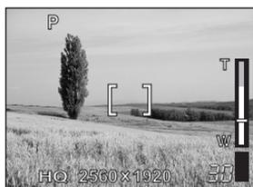
The white area of the zoom indicator indicates the optical zoom. If the [DIGITAL ZOOM] is set to [ON], a red area appears on the zoom indicator. When you reach the limit of the optical zoom, the digital zoom is enabled.
