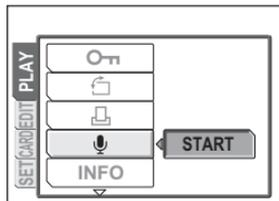
**2** Aim the camera microphone toward the sound you want to record and press to start recording.
