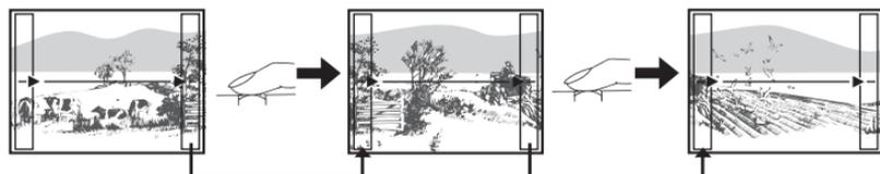
The part of the previous picture where it will be joined to the next picture does not remain in the frame on the edge of the screen. You have to remember what the part in the frame looked like and take the next picture so it overlaps. Compose your shots so that the right edge of the previous picture overlaps with the left edge of the next picture if you are connecting pictures from left to right (or vice versa if you are connecting pictures from right to left).
