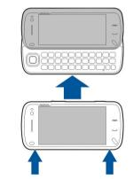
Your device has a full keyboard. To open the keyboard, push the touch screen up. In all applications, the screen rotates
