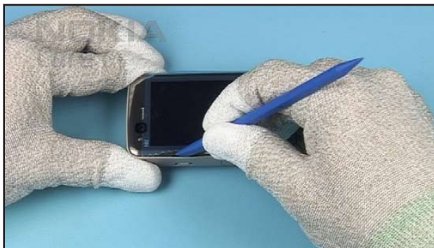
5. Move the opening tool to the shown place and open the next snap.
