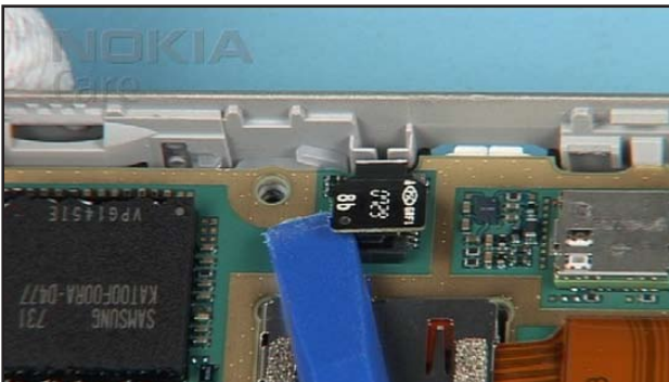
27. Carefully open the FLASH MODULE CONNECTOR.
