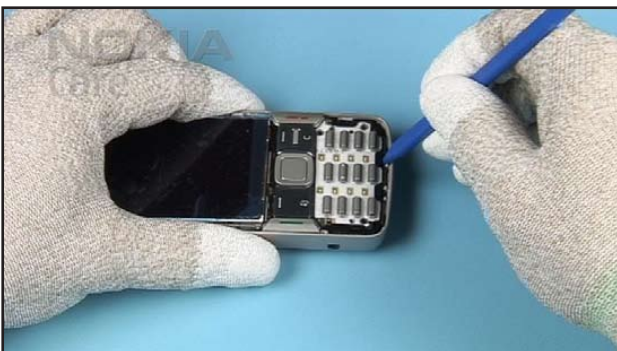
11. Unlock the bottom snaps of the UI Module.
