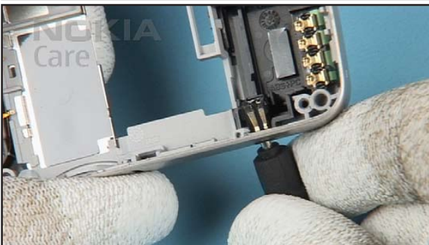
31. Remove the DC-JACK with the DC-Plug.
