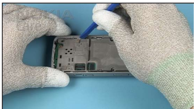
22. Unlock the MAIN FRAME ASSY starting at the shown side.
