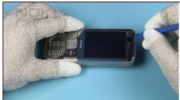
6. Now, open the snaps on the top of the WINDOW ASSY.
