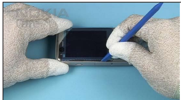
4. Use the SS-93 to open the snaps of the WINDOW ASSY.
