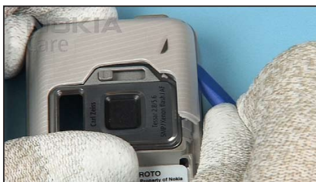
46. Gently unlock the D-COVER ASSY with the SS-93.
