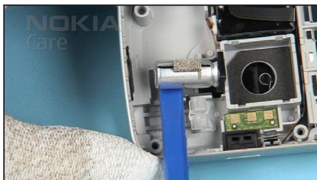
41. Carefully remove the CAPACITOR with the SS-93.
