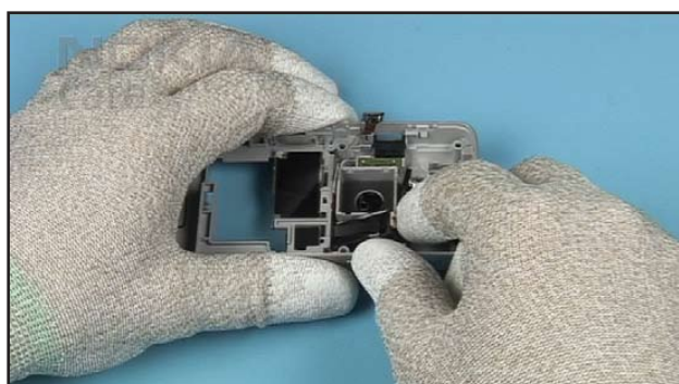
43. Carefully remove the FLASH MODULE...
