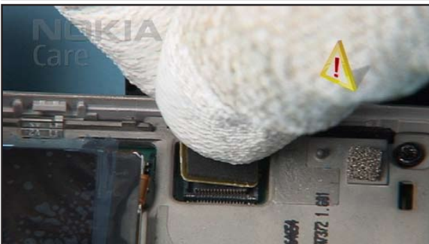
15. ...and very carefully open the UI MODULE connector.
