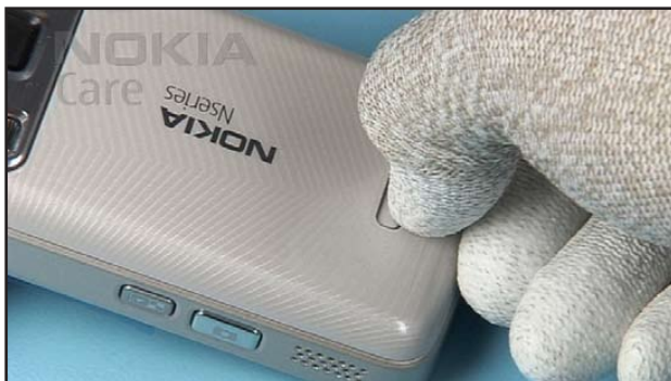
3. Unlock and remove the C-COVER ASSY. Remove the battery if inserted.
