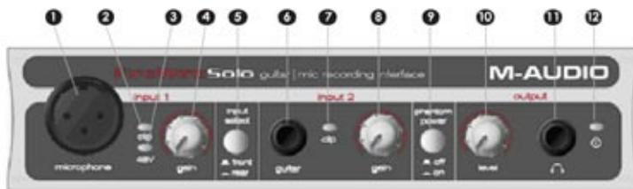
1. **Microphone Input** - Mic-level input on balanced XLR connector. This connector is only active when the Front/Rear Input Selector (5) is set to "Front" (OUT position). Input from this connector appears in your DAW software as a mono signal on the left side of the stereo input pair.
