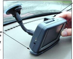
Then push back on unit until it snaps into place. You may need to lift the release tab slightly to engage unit.
