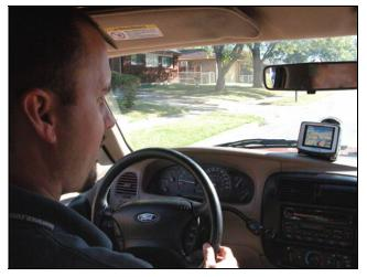
iWAY<sup>™</sup> 250c centered on a dashboard. This photo was taken at passenger eye level. Notice how the unit was placed so that it does not obstruct the view of the road ahead through the windshield.
