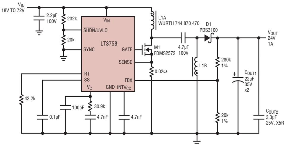
**Figure 5. A 18V-72V input, 24V/1A output SEPIC converter**
