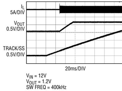
Figure 3. Start-up into a prebiased output
