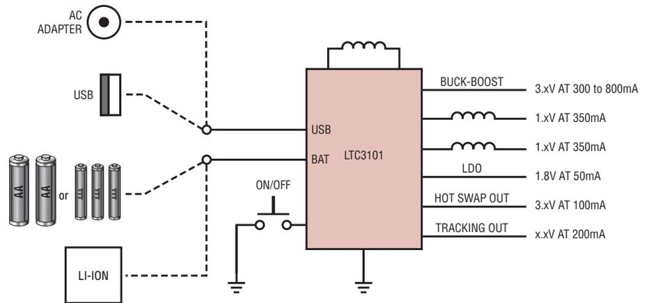
Figure 1. Six output rails, a low loss PowerPath and integrated pushbutton control
