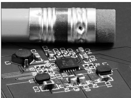
Figure 2. Complete portable power solution with a 16mm  $\times$  19mm footprint
