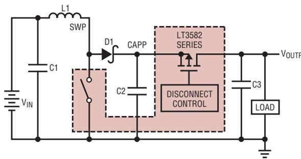
Figure 7. Output disconnect PMOS
