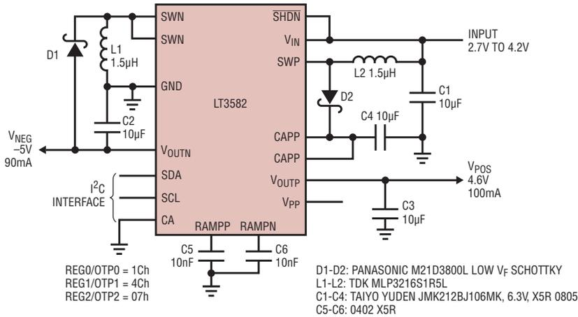
Figure 11. Tiny AMOLED power supply is 0.8mm (max) thin
