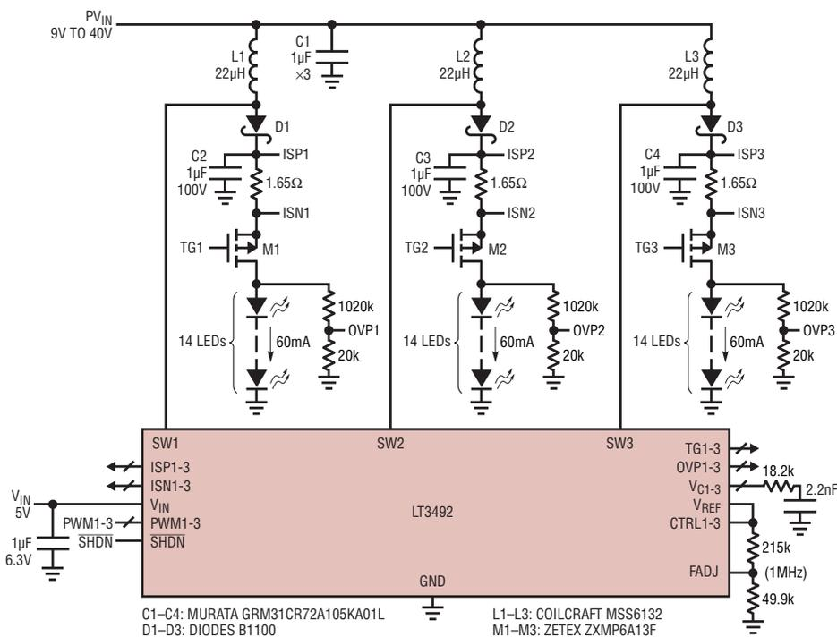
Figure 2. Triple boost mode 60mA x 14 LED driver
