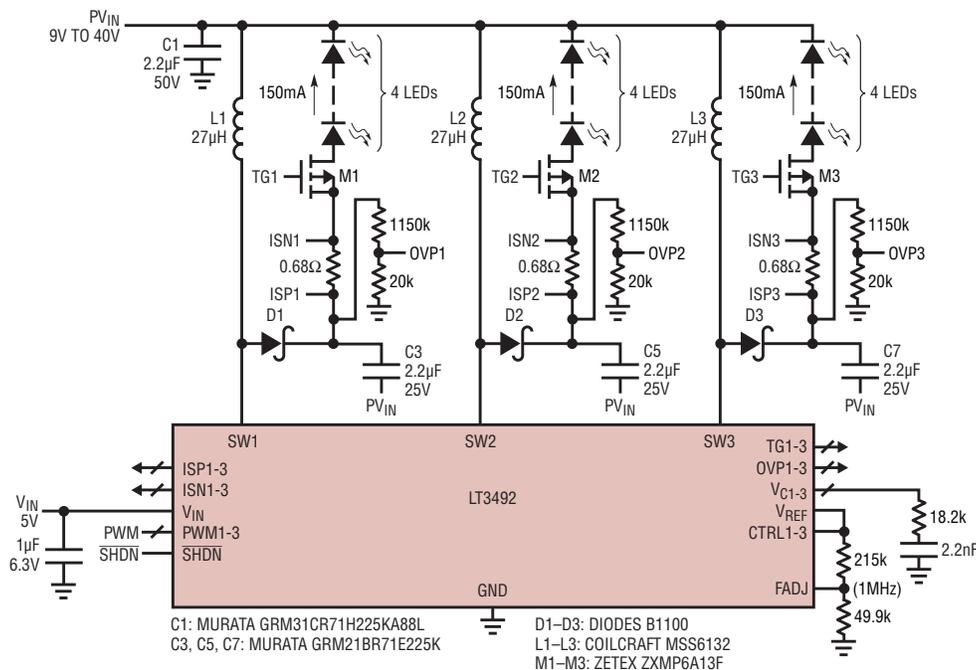
Figure 4. Triple buck-boost mode 150mA x 4 LED driver
