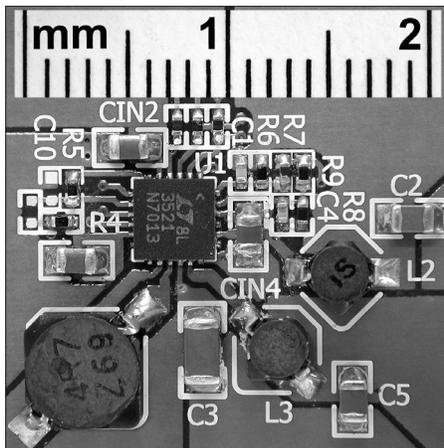
Figure 1. Buck-boost and buck converters occupy less than 0.5in<sup>2</sup> of board space.
