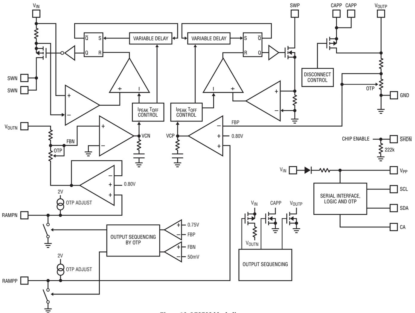
Figure 10. LT3582 block diagram
