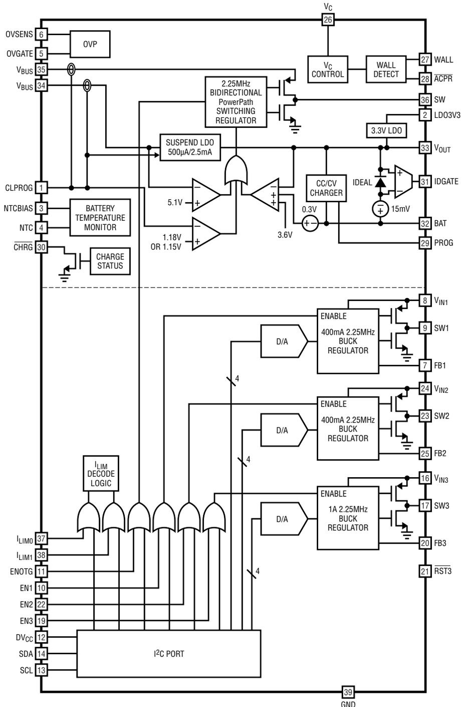
Figure 1. The LTC3576 combines USB charging and USB On-The-Go by using bidirectional DC/DC conversion from  $V_{BUS}$  to  $V_{OUT}$
