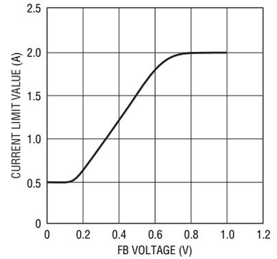
Figure 4. Current limit threshold foldback
