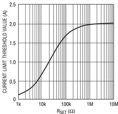
Figure 6. Current limit adjustment
