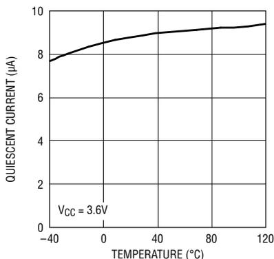
**Figure 4. Quiescent current vs temperature (not switching)**
