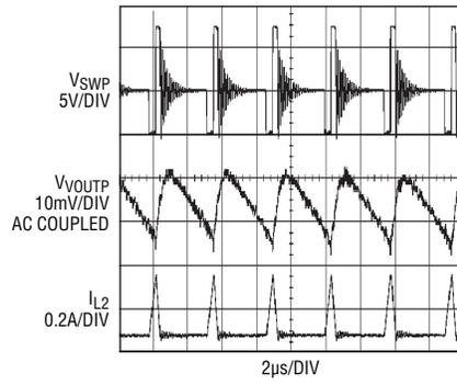
Figure 4. Switching waveforms at 10mA load for the boost application shown in Figure 2
