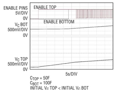
Figure 5. Charging with mismatched capacitors
