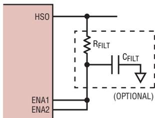
Figure 7. Sequencing the buck enables using the hot swap output rail
