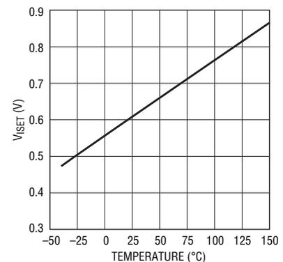
Figure 1.  $V_{ISET}$  vs temperature
