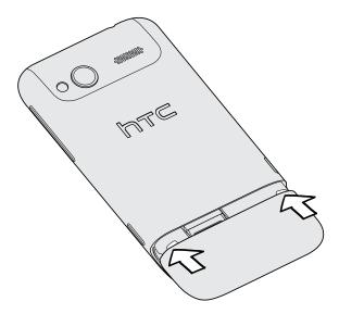
Your phone's antenna is placed underneath the bottom cover. We recommend that you make sure the bottom cover is correctly secured to the phone's back panel to get the best radio reception for your phone.
