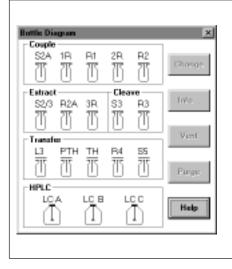
The Routine 4.0 sequencer methods require the bottle configuation shown. The reagents and solvents are purchased from Hewlett-Packard. These methods produce less than 1mL/cycle of liquid waste.
