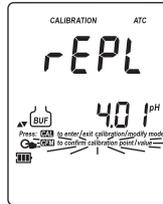
**Note:** The replaced buffer is not removed from the calibration list and can be selected for the next calibration.
