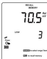
Press **Range** (HI 98150 & HI 98160) or **2nd** then **Mode** (HI 98140) and the instrument will display the next logged parameter as shown in the table below:
