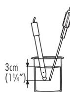
The LCD will show the pH measurement together with the temperature of the sample. In order to take more accurate pH measurements, make sure that the electrode and instrument is calibrated (see page 11 for details).
