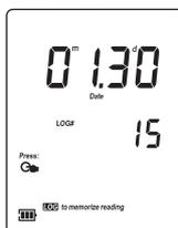
If there are less than 6 memory locations remaining, the “Lo” message will be displayed for a few seconds to alert the user, and then the available number of remaining logs is displayed on the LCD.
