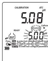
**Notes:** • Custom buffer value can be adjusted in a  $\pm 1.00$  pH window, around the set value.
