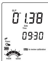
Press the **ARROW** keys to view the next calibration parameter (pressing the **▲** key):
