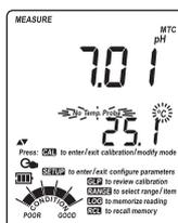
The "MTC" tag and ▲▼ arrow symbols light up on the LCD to indicate that the instrument is in MTC mode and the arrow keys can be used to enter the desired temperature value.
