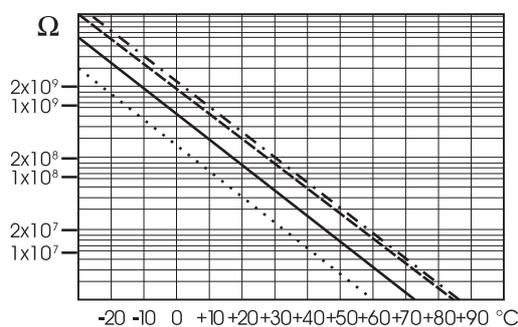
Since the resistance of the pH electrode is in the range of 50 to 200 Mohm, the current across the membrane is in the pico Ampere range. Large currents can disturb the calibration of the electrode for many hours.
