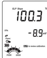
The GLP slope is the average of the calibration slopes; the percentage is referred to the ideal slope value. For example 59.16 mV/pH at 25 °C.
