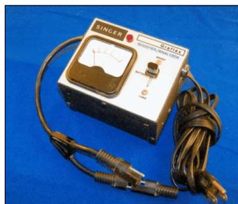
Analyzer into one unit (*GHQ* Vol. 13, Issue 3), the Booster/Analyzer for the new Graflex Electronic Flash System introduced in 1968 and 1970. It was specially designed for the Graflex Strobomatic 500 HV unit and the Graflex Strob 250, but with the Strobflash Adapter cord, Strobflash power Packs could also be tested.
