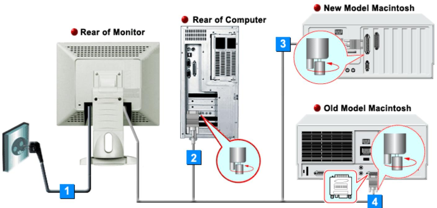
1. Connect the power cord for your monitor to the power port on the back of the monitor. Plug the power cord for the monitor into a nearby outlet..
