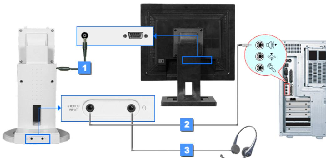
1. Connect the power cord of the multimedia stand to the multimedia stand power port on the back of the monitor.
