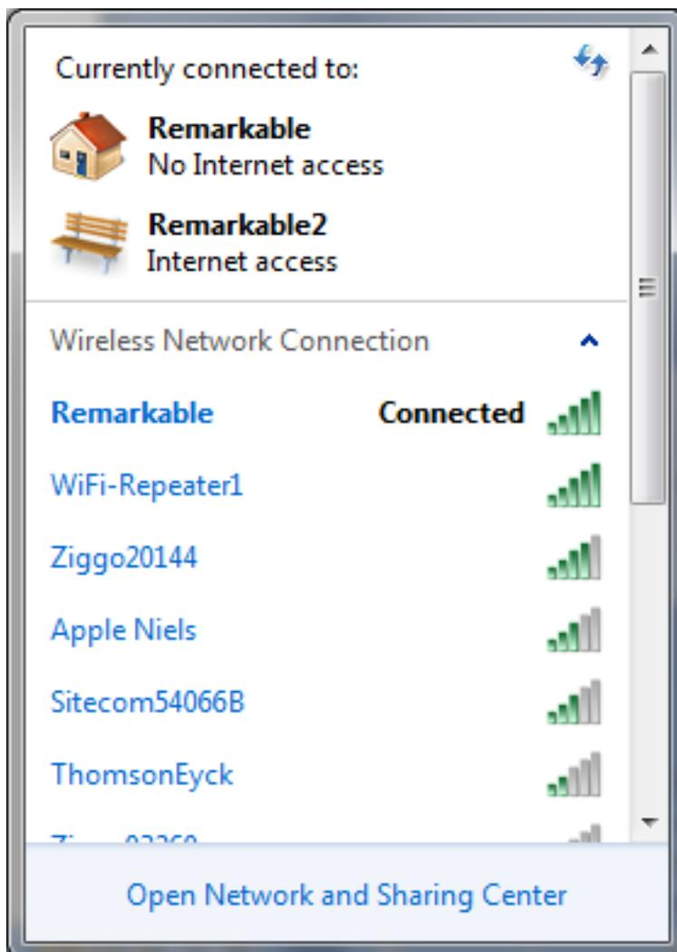
20. Select the “WiFi-Repeater1” network (click on it) and make sure the “Connect automatically” option is enabled.
