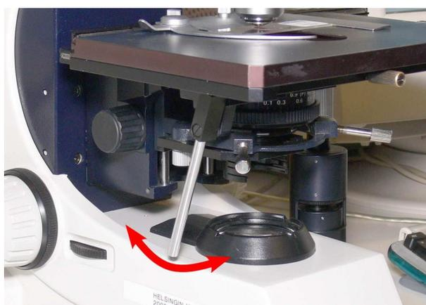
**Figure 4. Auxiliary condenser lens switch**
