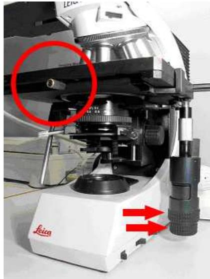
Figure 2. Adjustment wheels for stage control (arrows) and rotation lock (circle)
