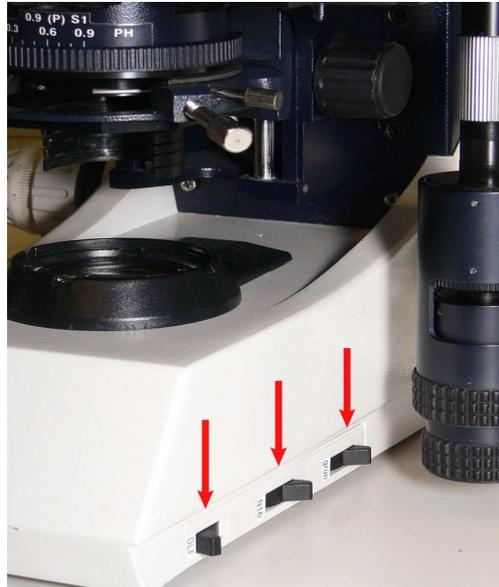
Figure 12. Filter controls marked with red arrows
