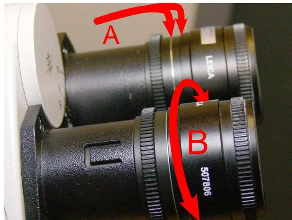
**Figure 6. Diopter adjustment. A, setting for 0 diopter; B, diopter adjustment**
