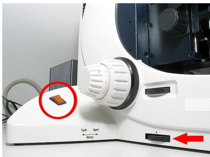
Figure 1. Power switch (red circle) and brightness control for halogen lamp (red arrow)
