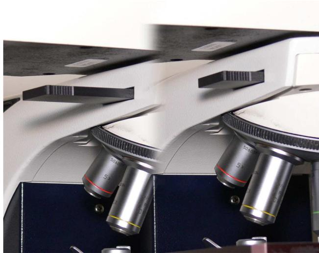
Figure 10. Analyzer for polarization contrast imaging
