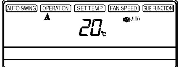
The temperature can be set within a range of 18°C~30°C by 1 °C.
