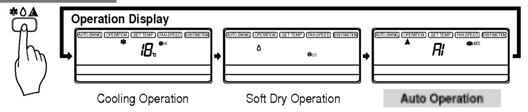
The temperature and fan speed are automatically set by the electronic controls based on the actual room temperature. If you want to change the set temperature, close the door on the remote control and press the Room Temperature Setting buttons. The cooler or warmer you feel, the more times (up to two times) you should press the button. The set temperature will then be changed. The temperature can be set within a range of -2~2 by 1 level.
