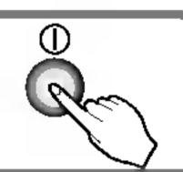
Open the door on the remote control. Press the PLASMA air purifying operation ON/OFF button. Operation will start when the button is pressed and stop when the button is pressed again.
