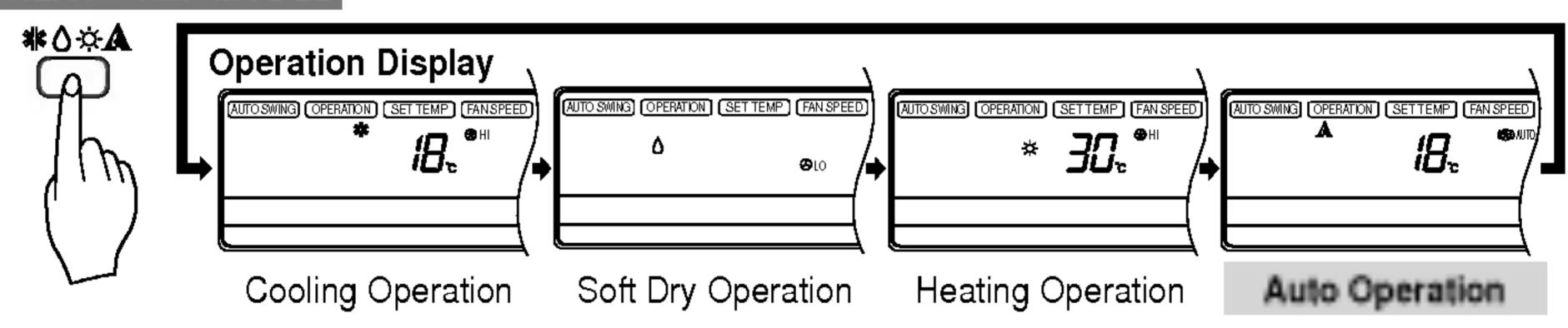
The setting temperature can be changed, when the set temperature button is pressed.
