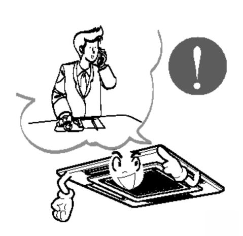
Do not let the air conditioner run for a long time when the humidity is very high and a door or a window is left open.
