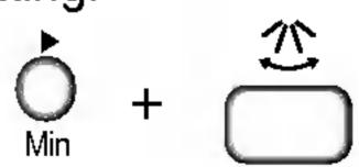
Press the left arrow button and Auto Swing button for three seconds in order to set the other two louvers. Next procedure is the same before.
