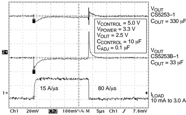
Figure 5. Transient Response Comparison between CS5253-1 and CS5253B-1
