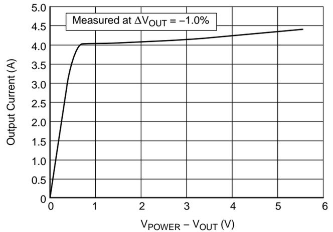
Figure 6. Output Current vs  $V_{POWER} - V_{OUT}$
