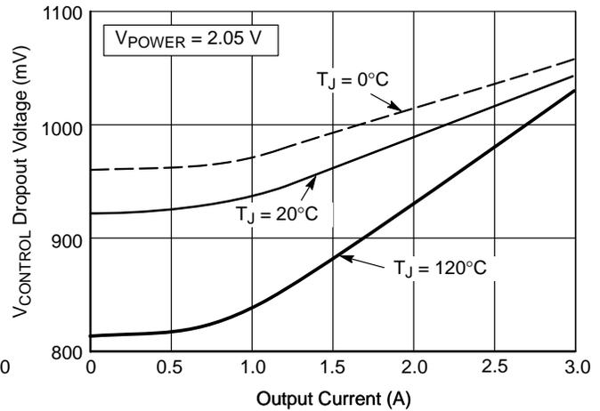
**Figure 12. VCONTROL Dropout Voltage vs Output Current**
