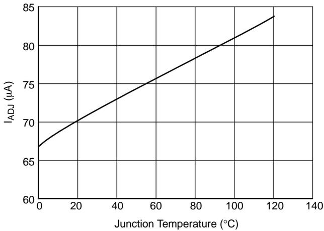
Figure 7. Adjust Pin Current vs Junction Temperature
