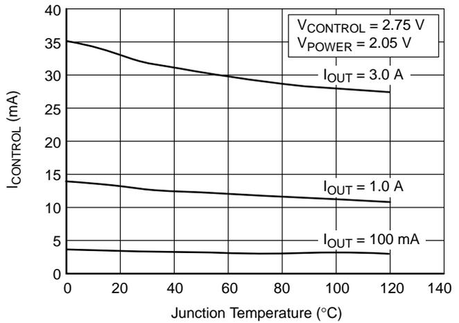
**Figure 16.  $V_{CONTROL}$  Supply Current vs Junction Temperature**
