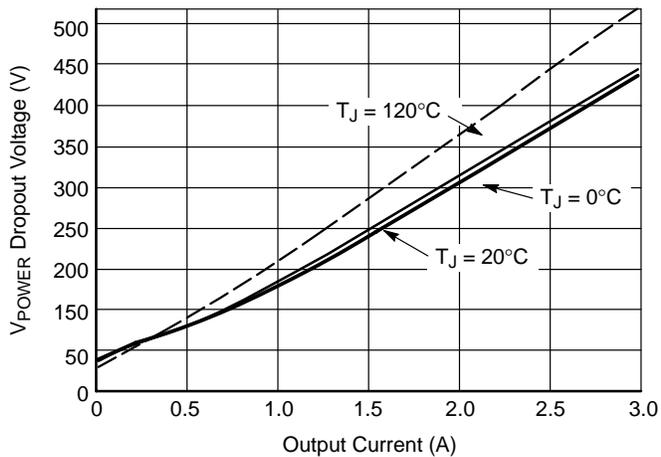
**Figure 13. VPOWER Dropout Voltage vs Output Current**
