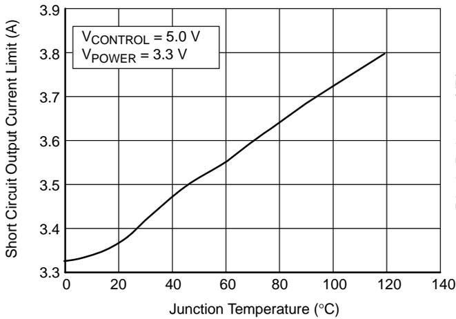
**Figure 9. Short Circuit Output Current vs Junction Temperature**
