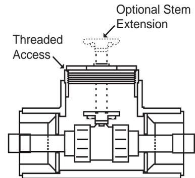
Using appropriate size daubers, apply cement to both Carrier pipe and extender coupling and to both Containment pipe and Valve Box Containment enclosure. Assemble immediately being sure to apply pressure to the opposite end extender coupling to seat Carrier connection.
