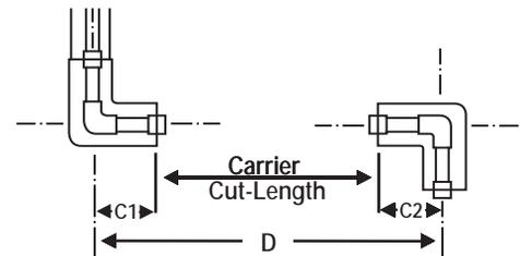
2. Containment Pipe Cut Length: Add the socket lengths for each of the two (2) connecting Containment fittings to the Carrier pipe cut length and cut the Containment pipe to that length.
