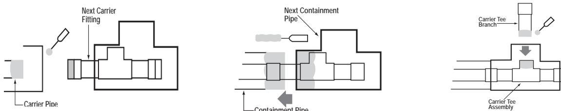
**Repeat Step 2 through 6** above to consecutively assemble each additional section of the Double Containment System. Finish with installation of an additional Termination Fitting. See following instructions on Closure Fittings or on Expansion Joints for joining Double Containment system sections which must meet.
