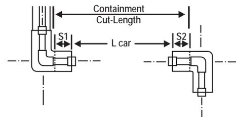
**COUPLING NOTE:** Regular couplings do not come with extenders. Where a continuation of a straight pipe run is made with a coupling on carrier or containment pipe, use the overall coupled length in the above calculations. Special allowances should also be made for Closure Fittings and Expansion Joints in determining cut lengths.
