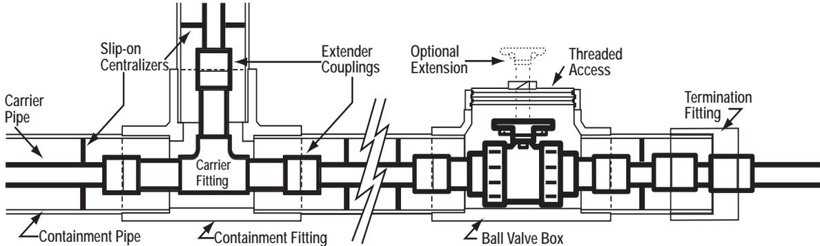
Successful installation requires proper design and planning of system layout, a basic understanding of how Spears® double containment fitting design works, and specific attention to a proper sequence of general assembly. This manual is designed as a general guide and may not address all situations encountered. Due to the variety of selected Carrier/Containment combinations some design variations may occur.
