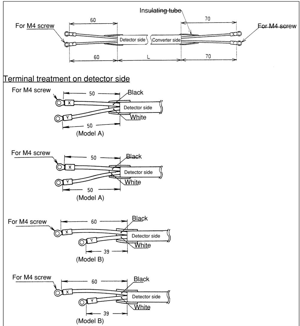
Figure 2-9 Excitation Cable Construction
