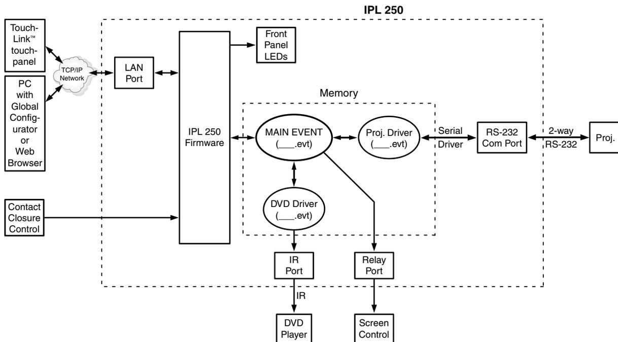
The IPL can be configured completely via Global Configurator software. Once you have set up how you want it to work (assigned drivers to ports, configured relays and contact closure input, and set up IP addresses and functions), that information is saved to a project file that is uploaded into the IPL.
